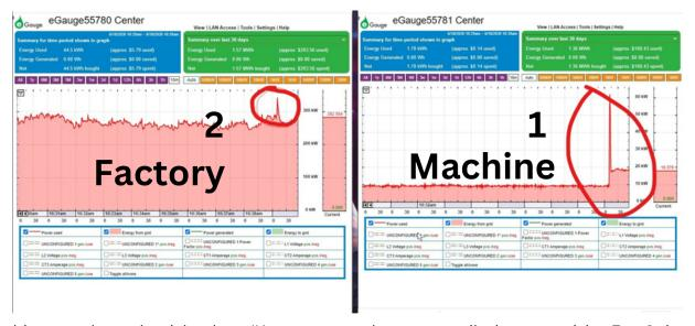
In this example on the right chart #1, we can see the severe spike in power rising 7 to 8 times higher causing a large voltage drop to surrounding equipment and driving the Factory #2 over it's demand limit, triggering additional power costs. You pay the power company extra for your problems that cause downtime and damage.
